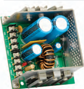
12 VDC, 5 A Power Supply PCBA
