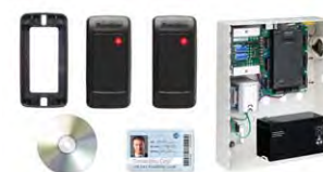
AC-225IP E/L 2-Door Kit (230/110 VAC Transformer)
