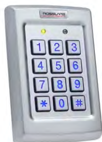
Anti-Vandal Backlit PIN Standalone Controller
