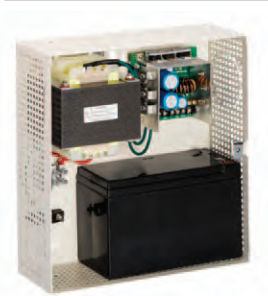
12 VDC, 5 A Power Supply Unit (battery not included)
